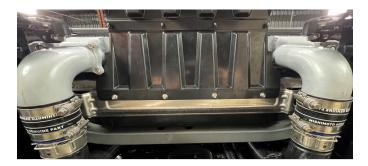
**68.** Remove the stock intercooler quick disconnect adapters and boots. (4x MM1533-92 clamps)
