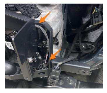
**56.** Unseat the connector from the driver-side of the radiator grille shutter assemble.
