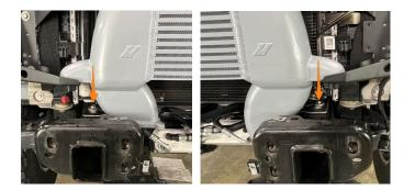
**35.** Install 2x MM2392-03 using the provided 12mm length bolts. Do not fully tighten the bolts as the brackets' final position will be adjusted in a later step. [4x HF6X1.0-12A]
