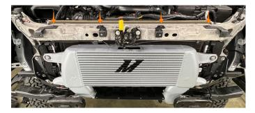
**37.** Install MM1867-03 and -04 to the brackets previously installed in step 35 using the provided pop clips. [4x MM930]
