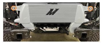
**34.** Pull outward on the upper intercooler mounting bracket, ducting, and foam assembly until the ½" mounting holes align with the threaded holes in the frame. Once aligned, use the original fasteners to secure it in place. (2x 15mm bolts) (Images on next page)
