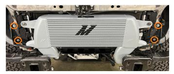
**33.** Secure the intercooler to the brackets using the provided 12mm bolts. (2x HF8X1.25-25A)
