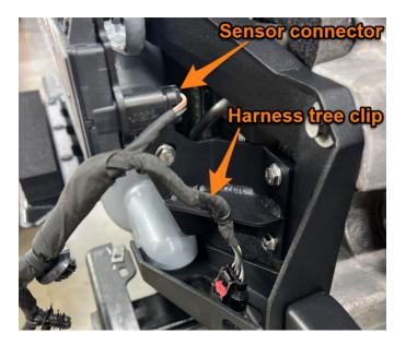
**52.** Secure the intercooler grille shutter harness to the MM2392-05 bracket using the harness tree clips. Route the harness as shown above.
