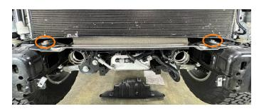
**20.** Remove the large adhesive backed foam strip from the upper intercooler bracket using a heat gun. Once removed, clean off any residual adhesive from the bracket.
