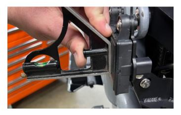
**50.** Using a square with a bubble level, adjust the MM2420-02 bracket until level. Once level, tighten the bolts.
