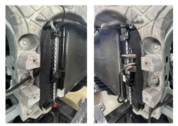
27. Apply the two 110mm long pieces of MM1280-11 adhesive backed foam to the back sides of MM2392-01 and MM2392-02 in the locations shown. (2x 110mm long MM1280-11)
