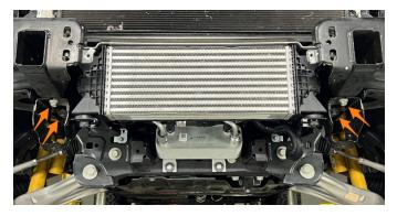
**18.** Disconnect the intercooler inlet and outlet, then remove the intercooler from the vehicle.
