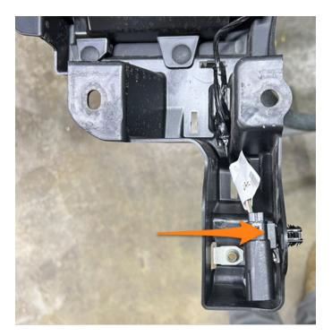
**57.** Remove the connector tree clip from the connector using a panel tool or flat head screwdriver.
