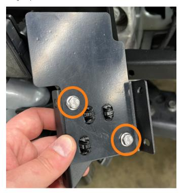
**54.** Install the MM2392-05 bracket to the driver-side intercooler bracket using the provided hardware. Reconnect the intercooler grille shutter harness to the vehicle body harness and attach the connector tree clip to the MM2392-03 bracket as shown in the above image. (2x HF6X1.0-12A) **\*If your vehicle is equipped with Active Cruise Control, skip 55.**
