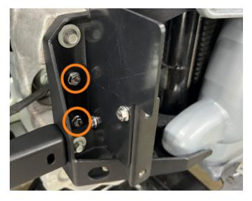
**63.** Install the MM2392-11 bracket to the MM2392-04 and -05 brackets using the provided hardware. Align the bottom of the brackets, then tighten the bolts. (2x HF6X1.0-12A)
