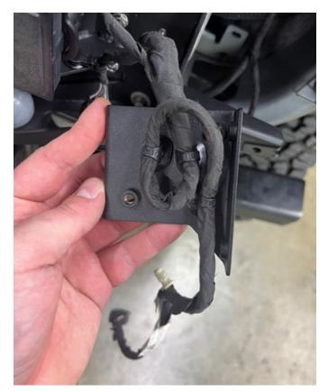
**53.** Attach the MM1867-06 duct panel to the MM2392-05 bracket using the provided hardware. (2x HF6X1.0-12A)
