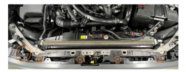
**04.** Locate the front two rotating fasteners securing the fender flares in place and turn them 90 degrees, then pull outward to partially remove them. Do this on both sides.
