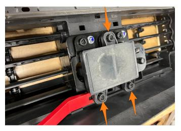
**45.** Remove the 3x plastic bushings from the sensor by pushing the tabs inward while applying some downward pressure, then push the bushings out of the sensor brackets.
