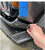
**06.** Unseat the front fascia from the clips that secure it to the grille support structure. Once fully unseated, remove the front fascia from the vehicle.
