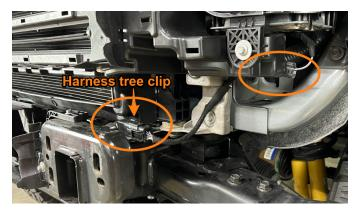
**11.** Remove the intercooler active grille shutter assembly from the vehicle. [4x 8mm bolts]
