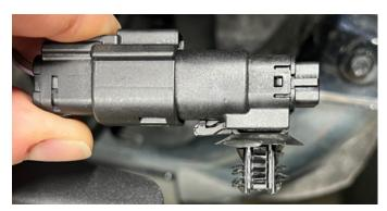
**60.** Secure the radiator grille shutter motor connector to the body of the vehicle in the location shown above.
