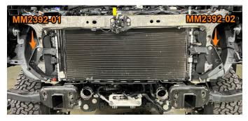
**29.** Remove the 4x 10mm bolts securing the lower section of the passenger-side intercooler end tank in place, then remove the lower section of the end tank from the intercooler.
