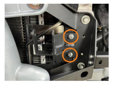
**48.** Fasten the MM2420-01 bracket and sensor assembly to the MM2420-02 bracket using the provided hardware. (1x HF6X1.0-14 and 1x HF6X1.0-50)
