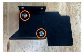
62. Install the MM2392-04 bracket to the passenger-side intercooler bracket using the provided hardware. (2x HF6X1.0-12A) (Image on top right)
