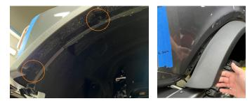
**05.** Pull outward on the rear corners of the front fascia to unseat it from the clips that secure it to the fenders. Do this on both sides.
