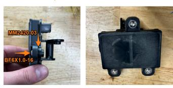
**47.** Install the MM2420-02 bracket to the driver-side intercooler mounting bracket using the provided hardware. (2x HF6X1.0-14)
