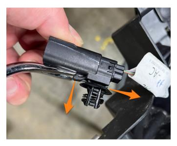
**58.** Install the connector tree clip onto the provided radiator grille shutter motor connector.
