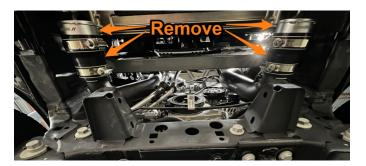
69. Using the MM4634-01 extended boots, connect the Mishimoto intercooler piping to the inlet and outlet of the intercooler.(4x MM1533-92 clamps)
