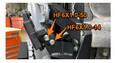
**63.** Using a square with a bubble level, adjust the sensor pivot angle until it is level. Once the sensor is level, tighten the bolts.
