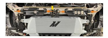
**52.** If your vehicle is equipped with the modular bumper, fasten MM1867-02 to the upper intercooler bracket, ducting, and foam assembly using the provided pop clips. (4x MM930). \*Proceed to step **53** if your vehicle is not equipped with the modular bumper.
