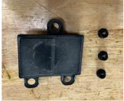
**60.** Fasten the adaptive cruise control sensor to the MM2420-01 bracket using the provided hardware and spacers. (3x BF6X1.0-16 and 3x MM2420-03 spacers)
