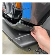
**06.** Unseat the front fascia from the clips that secure it to the grille support structure. Once fully unseated, remove the front fascia from the vehicle.
