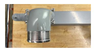
**44.** Install the provided grommets and bushings on to the intercooler. [2x MM1281-15 and 2x MM1742]
