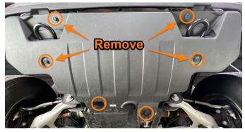
17. Remove the lower intercooler brackets. (4x 15mm bolts)
