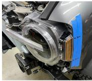
**54.** Carefully remove the wiring harness from the intercooler grille shutter assembly.
