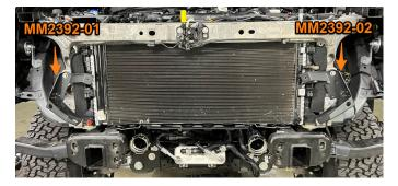
**43.** Remove the 4x 10mm bolts securing the lower section of the passenger-side intercooler end tank in place, then remove the lower section of the end tank from the intercooler. (Image on top right)
