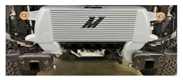
48. Pull outward on the upper intercooler mounting bracket, ducting, and foam assembly until the  $\frac{1}{2}$ " mounting holes align with the threaded holes in the frame. Once aligned, use the original fasteners to secure it in place. (2x 15mm bolts)
