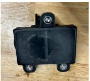
**61.** Install the MM2420-02 bracket to the driver-side intercooler mounting bracket using the provided hardware. (2x HF6X1.0-14)
