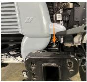
**49.** Install  $2x \, MM2392-03$  using the provided  $12mm \, length \, bolts$ . Do not fully tighten the bolts as the brackets' final position will be adjusted in a later step. [ $4x \, HF6X1.0-12A$ ]
