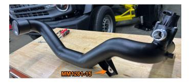
**29.** Using the provided clamps and turbo boot, install the Mishimoto hot-side intercooler pipe. Do not tighten the clamps, this will be done later. Reconnect the bypass valve hose and electrical harness. [MM4623-01, MM1533-66, and MM1533-79]
