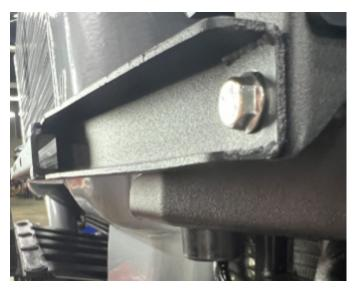
**78.** Install the MM2392-10 bracket to the MM2392-04 and -05 brackets using the provided hardware. Align the top of the brackets, then tighten the bolts. (2x HF6X1.0-12A)
