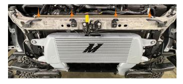
**51.** Install MM1867-03 and -04 to the brackets previously installed in step 35 using the provided pop clips. [4x MM930]
