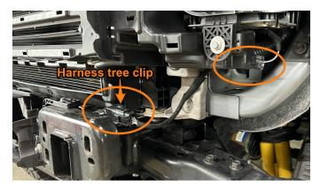
11. Remove the intercooler active grille shutter assembly from the vehicle. [4x 8mm bolts]
