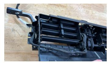
**55.** Push the provided cavity plugs into the open cavities located on the back side of the provided intercooler grille shutter motor connector.
