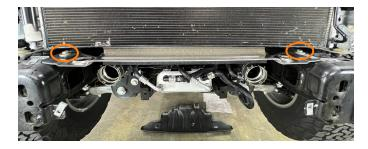
**34.** Remove the large adhesive backed foam strip from the upper intercooler bracket using a heat gun. Once removed, clean off any residual adhesive from the bracket. (Images on next page)
