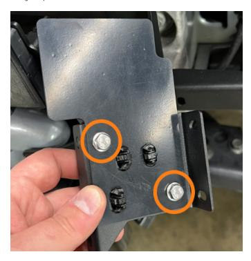
68. Install the MM2392-05 bracket to the driver-side intercooler bracket using the provided hardware. Reconnect the intercooler grille shutter harness to the vehicle body harness and attach the connector tree clip to the MM2392-03 bracket as shown in the above image. (2x HF6X1.0-12A) \*If your vehicle is equipped with Active Cruise Control, skip 69.
