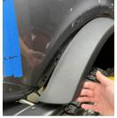
**05.** Pull outward on the rear corners of the front fascia to unseat it from the clips that secure it to the fenders. Do this on both sides.
