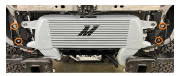
**47.** Secure the intercooler to the brackets using the provided 12mm bolts. (2x HF8X1.25-25A)
