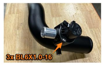
**28.** Install the provided grommet onto the Mishimoto hot-side intercooler pipe. (MM1281-15)
