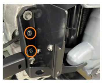
77. Install the MM2392-11 bracket to the MM2392-04 and -05 brackets using the provided hardware. Align the bottom of the brackets, then tighten the bolts. (2x HF6X1.0-12A)
