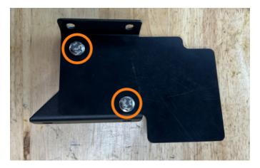
**76.** Install the MM2392-04 bracket to the passenger-side intercooler bracket using the provided hardware. (2x HF6X1.0-12A)
