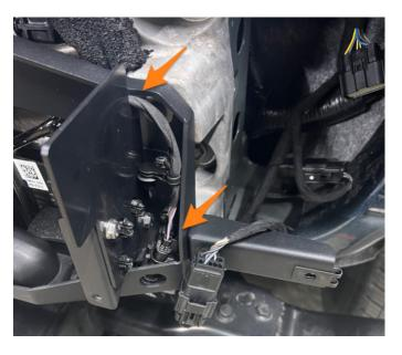
**70.** Unseat the connector from the driver-side of the radiator grille shutter assemble.
