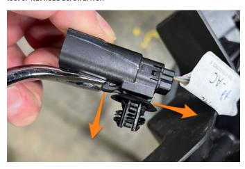
**72.** Install the connector tree clip onto the provided radiator grille shutter motor connector.
