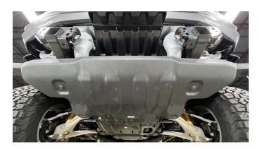
**91.** Guide the front bumper back onto the vehicle, ensuring that the lower intercooler ducting slides into the upper area of the bumper.
