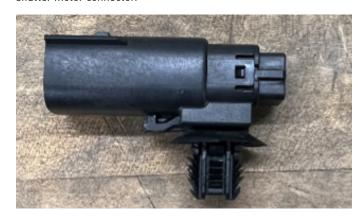
**73.** Connect the provided radiator grille shutter motor connector to the vehicle body harness.
