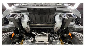
90. Reinstall the front skid plate. (Image on right)
