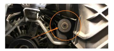
**10.** Remove the 1X 13mm bolt holding the electrical harness to the right-side valve cover near the oil fill cap and then remove the 2X E8 External Torx bolts holding the oil fill cap assembly and remove. Use a paper towel or tape to cover the hole to ensure nothing falls into the engine.
