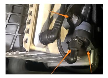
**08.** Remove the MAP sensor electrical connector and loosen the clamp connecting the throttle body coupler to the intake manifold, on the throttle body side. Repeat on other intercooler.
