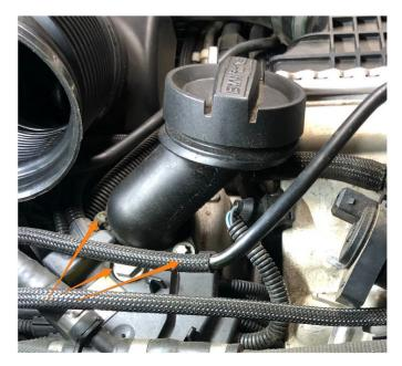
**11.** Remove factory charge pipes from the vehicle. There will be two identical Mishimoto transition couplers that will fit on the turbo outlet. Install 1X transition coupler on each turbo and install and tighten 1X 52-75mm worm gear clamp securing the coupler to the turbo. Repeat on other turbo. Install another 52-75mm clamp onto the other end of the coupler and push the long, straight end of the charge pipe into the coupler. Repeat with other charge pipe but leave loose for now.
