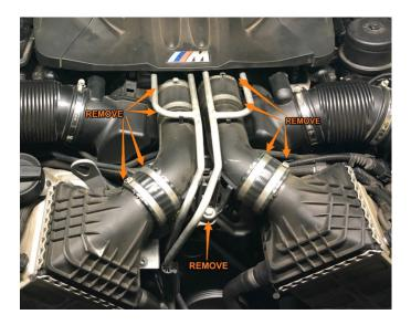
**06.** Remove the 2X water lines from each intercooler (4 total), using a pick tool to release the lock and pull the fittings and lines away from the coolers. Remove the 1X vent line from each intercooler (2 total) in a similar fashion.
