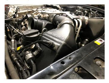
**21.** Reinstall the Oil fill tube. Inspect the O-ring before installation and replace if necessary (BMW PN. 07119906276). Tighten both E8 Torx bolts to approx. 9 ft-lbs. Don't forget to reinstall the 13mm bolt securing the engine harness to the valve cover.
