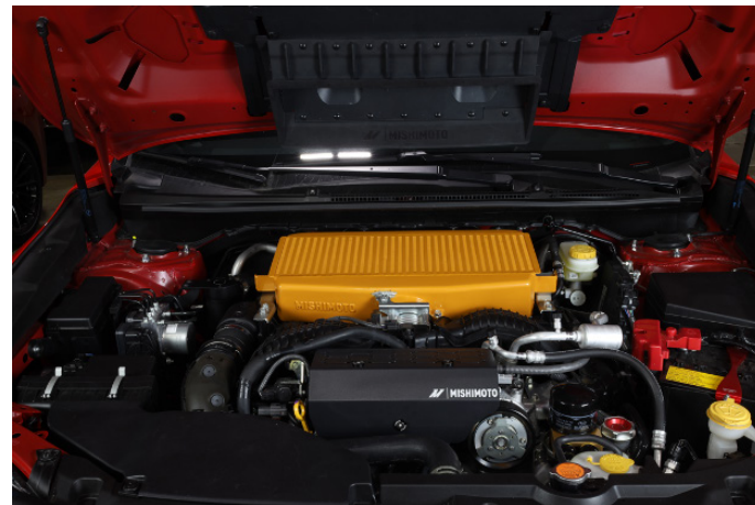
Figure 2: 2022 WRX with Mishimoto top mount intercooler upgrade installed.
