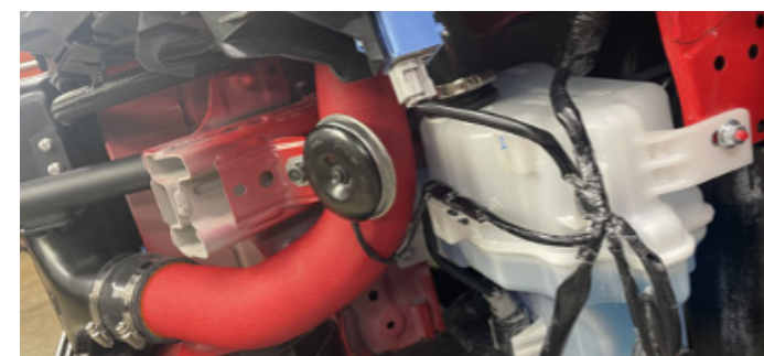
Figure 9: Side view of the intercooler and intercooler outlet pipe shows the tight precise fitment of the charge pipe to allow the retention of the side-front impact supports.
