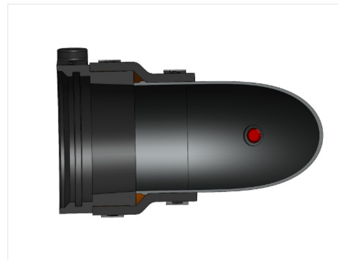
Figure 7: This cutaway of the throttle body connection shows the inlet matches the internal diameter of the charge pipe and an outlet that matches the internal diameter of the throttle body to promote smooth flow.
