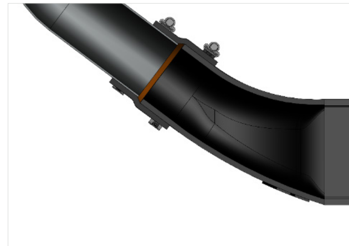
Figure 6: Intercooler inlet and outlet have a matched internal diameter to promote smooth flow.
