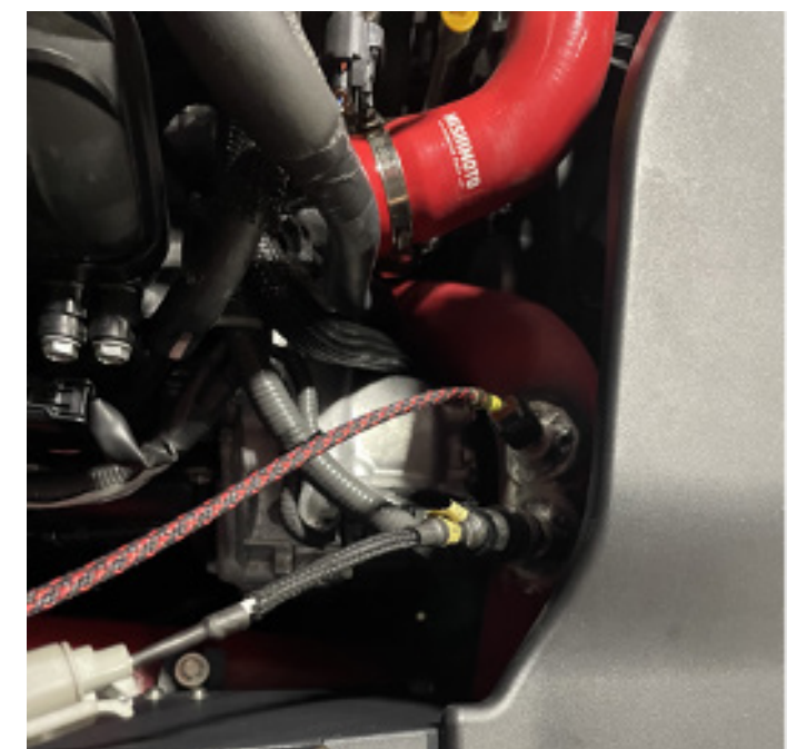
Figure 14: Temperature and pressure sensors located in the turbo outlet charge pipe, to accurately measure the air leaving the turbocharger.
