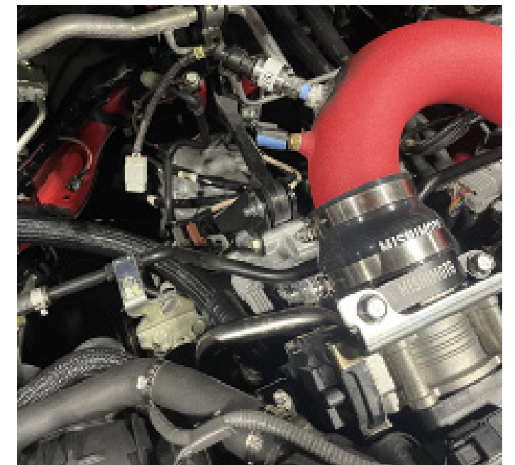
Figure 13: Temperature and pressure sensors located in the charge pipe, close to the throttle body.
