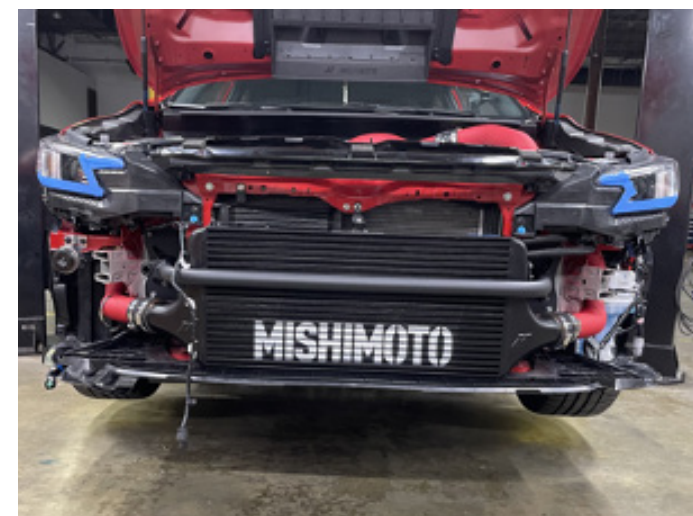
Figure 8: Front view of the intercooler system shows the included bumper beam and the retention of the side-front impact supports diameter to promote smooth flow.
