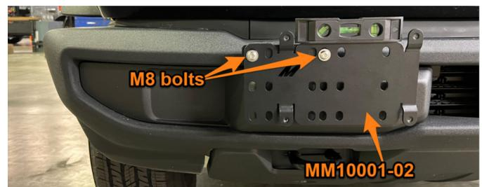
6. Fasten the front license plate to MM10001-02 with the provided M6 bolts.
