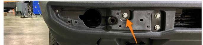
3. Fasten the MM10001-01 bracket to front bumper using the 15mm bolt removed in the previous step. Torque the bolt to 81 lb/ft.
