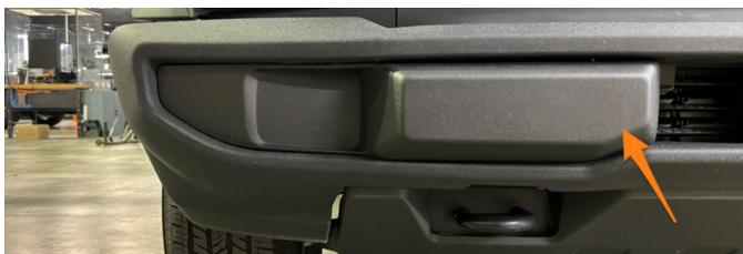
2. Remove the outermost 15mm bolt from the front bumper.
