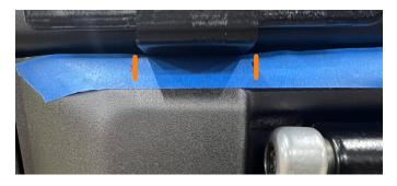
5. Remove the trim panel from the bumper and transfer the markings to the back side as shown. Using a file and sandpaper, trim the marked area.
