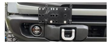
**9.** Fasten the front license plate to MM10001-02 with the provided M6 bolts.
