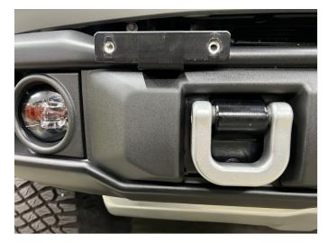
8. Fasten MM10001-02 to MM10048-01 in the desired orientation using the provided M8 bolts. A level should be used to ensure a nice, clean installation.
