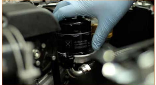
7. Install the Mishimoto sandwich plate. Make sure to lubricate the O-ring with oil to create a proper seal.
