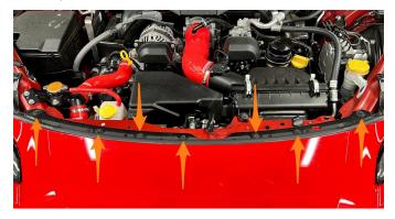
05. Reach around the back of the bumper here and pull straight out and away from the vehicle until the bumper pops free. Work up toward the headlight, releasing all the clips. Repeat for the other side and remove the bumper from the vehicle.
