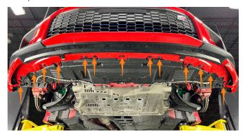
**04.** Using a 10mm socket, remove the 5 bolts and use a trim tool to remove the 2 pop clips. Remove the black metal/rubber trim piece.
