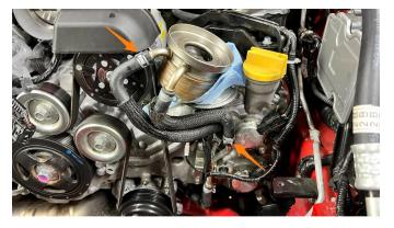
**19.** Loop the remaining coolant hose back to the other pipe and secure it with the hose clamp.
