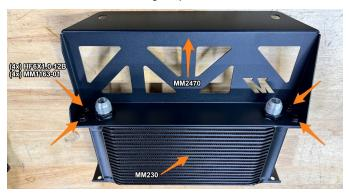
10. Install hose 1 and 2 onto the oil cooler in the orientation shown.
