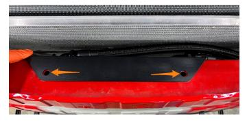
12. The 4 provided self-tapping screws can be used to fasten the oil cooler to the plastic reinforcement piece if a more secure installation is required.
