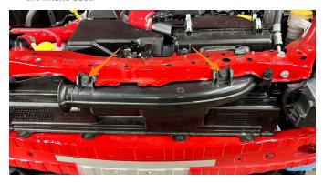
**07.** Using a trim tool, remove the 6 pop clips then remove the cowl piece.
