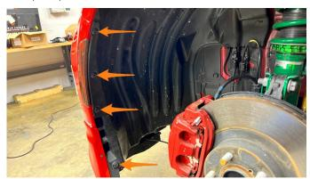
**02.** Pull back the liner and unplug the side marker light plug. Repeat on the other side of the vehicle.
