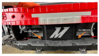
**13.** Feed the oil cooler lines under the crash bar and under the driver-side headlight as shown.
