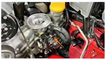
20. Place the thermostatic sandwich plate over the oil filter housing O-ring side down then place the cup over top of the plate as shown. Thread the longer M20 center bolt into the housing and tighten using a 27mm deep socket.
