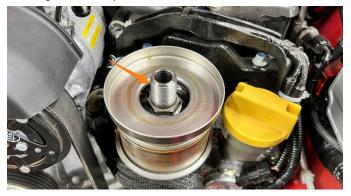
**18.** Use channel locks to loosen the 2 clamps and disconnect the coolant hoses from the tubings at the 2 location shown. Remove the stock oil cooler.
