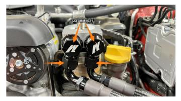
23. This step is optional but recommended to prevent the engine from running dry on the first startup. Remove the left side AN fitting and push the outlet hose of a fluid transfer pump into the fitting. Use the pump to prefill the oil cooler and lines with engine oil until you see it come out of the hole in the sandwich plate. Once filled, remove the hose, and reinstall the AN line and the oil filter.
