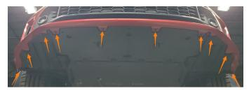
2. Disengage the clips that attach the bumper to each wheel liner by inserting a flathead screwdriver. Then, using a flathead screwdriver or pop clip pliers, remove the two (2) pop clips in each wheel well that attach the bumper to the wheel liner.
