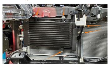
12. (Optional) Mark the shroud that was removed in step 8 in the locations shown in the photo below and cut a hole using a 1-1/4" hole saw or aviation snips. These holes will allow the oil line fittings to pass through the shroud and connect to the cooler. This step is optional; the shroud can be left off the vehicle if you prefer not to cut the shroud. A replacement shroud can be purchased from a Toyota dealer. The shroud is Toyota part number 16593-18030.
