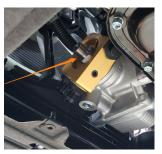
17. Using an adjustable or -10B AN wrench, attach the AN lines from the cooler to the sandwich plate fittings, as shown in the photo below. Angle the sandwich plate towards the front of the vehicle and tighten the center bolt to 30 lb-ft with a 27mm socket. Then, reinstall the oil filter onto the center bolt.
