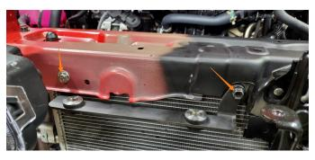
11. Install the lower mounting bracket to the hood latch support using the two (2) supplied 20mm long M6 bolts, M6 washers, and M6 nyloc nuts. Then attach the cooler to the mounting brackets using the three (3) supplied M8 bolts.
