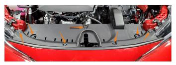
**4.** Using a 10mm socket, remove the three (3) bolts securing the top of the bumper to the vehicle.
