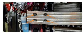
**8.** Using a flathead screwdriver or pop clip pliers, remove the pop clip and disengage the clip connecting the plastic shroud to the air duct. Then disengage the clip connecting the shroud to the radiator and remove the shroud from the vehicle.
