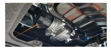
16. Using a 25mm wrench, install the supplied sandwich plate fittings to the sandwich plate. Then, loosely install the sandwich plate onto the engine with the supplied center bolt. The side of the sandwich plate with the gasket should be against the engine.
