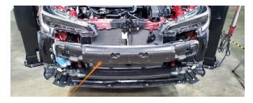
7. Using a 10mm socket, remove the nut that attaches the bracket to the bottom center of the crash bar. Then, unclip the plastic wire harness mount from the top of the crash bar. Then, using a 14mm socket, remove the four (4) bolts on each side of the crash bar and remove the bar from the vehicle.
