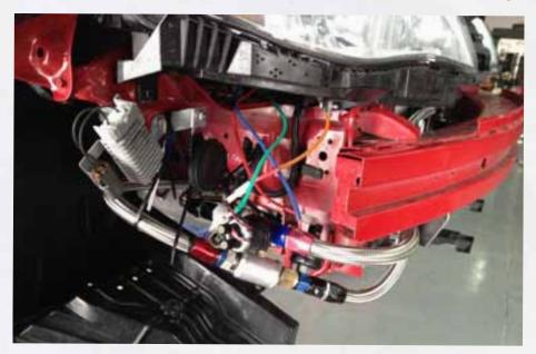
A thermocouple was mounted in the front grille with no obstructions so that ambient air temperatures could be measured.
