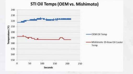
The graph above compares the temperatures of the oil returning to the engine with and without the oil cooler installed. A drop in temperature of roughly 36°F occurs when the STI is equipped with the Mishimoto 19-row oil cooler.
