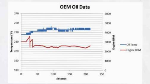
At cruising speeds, the OEM oil temperature is around 223 degrees F.
