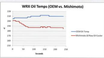
At cruising speeds, the oil temperatures coming into the cooler are around 200-215°F. The graph on the left shows that, under cruising conditions, the Mishimoto oil cooler reduced temperatures by more than 25°F and approximately 20°F on average over stock.
