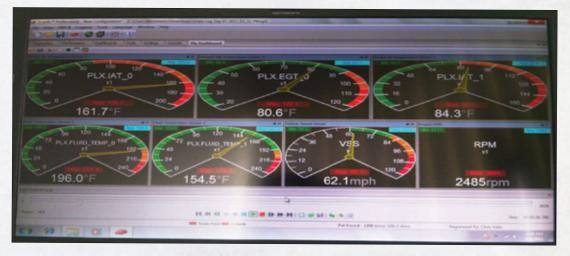
Fluid temperatures were taken from both the inlet and outlet of the 10-row oil cooler using a Mishimoto oil sandwich plate with PLX fluid temperature sensors. Oil pressure was also tested to ensure no dramatic pressure drop occurs when installing the oil cooler.
