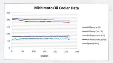
The graph on the left shows that the Mishimoto oil cooler loses only 1-2 psi of pressure compared to the stock setup.
