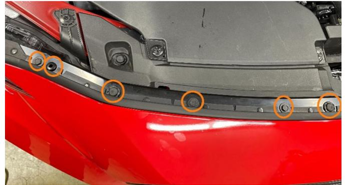
**07.** Pull the bumper from the fender on each side by pulling the bumper outwards. Repeat for other side of the vehicle. Then, pull the bumper away from the vehicle just enough to remove the fog light electrical connectors on each side. Then pull the bumper away from the vehicle. It may be beneficial to have a second person to help handle the bumper removal.
