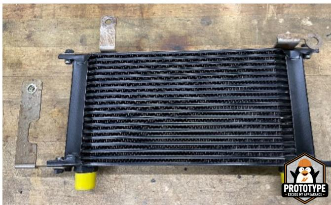
**11.** Prepare one of the included M8 bolts and install the oil cooler. Use the m8 bolt to hang the oil cooler from the factory hole (Bolt #1 in picture). Leave this bolt loose. Then, install the included M6 bolt through the core support and into the lower oil cooler bracket (bolt #2). Leave this bolt loose for now.
