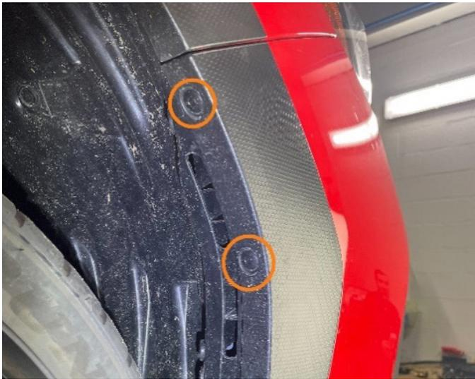
**06.** Remove the 5x pop clips, and 6x 10mm bolts at the top of the bumper and remove the black metal trim piece on top of the bumper.
