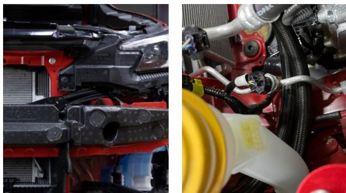
**17.** Install the oil lines onto the banjo bolts and then install the banjo bolts onto the sandwich plate. The shorter of the two lines goes to the passenger side of the sandwich plate and the longer line goes to the driver's side.
