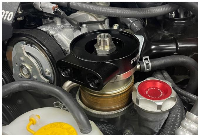
**14. THERMOSTATIC ONLY:** Remove the oil filter and then remove the 24mm center bolt holding the oil filter assembly to the engine. Remove the clamps and coolant hoses attached to the oil filter housing and remove from the vehicle.
