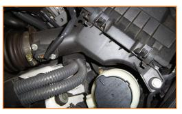
**4.** Remove the 10mm head screw on the LEFT side frame rail for the A/C system line.
