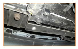
2. Unplug the fan connectors on the right side of the vehicle and remove the wire clip that attaches the fan wiring to the radiator fan shroud.
