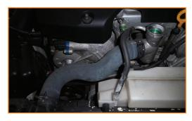
**7.** Turn the upper radiator securing points to unlock and remove the mounts.
