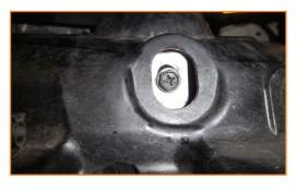
3. Install the upper mounting clips and turn to lock position. Install the fan shroud, coolant overflow tank, upper radiator hose, lower radiator hose, fan plugs, A/C line bracket and air boxes. Installation is reverse of removal.
