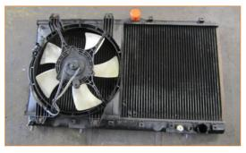
2. Reinstall the fans using the (8) 12mm bolts and reinstall the two sensors into the Mishimoto radiator. Apply Teflon tape to the threads of the sensors to prevent leaks.
