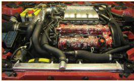
**6.** Reinstall and tighten the negative terminal of the battery. Refill coolant, check for leaks, and bleed out air by turning the vehicle on and squeezing the upper and lower radiator hoses. Lower vehicle and conduct a road test. Check for leaks in the coolant system. Once no leaks are determined, reinstall the (14) 12mm bolts and (4) plastic clips for the lower splash shield.
