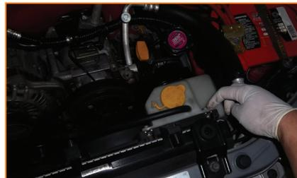
5. Remove the 10mm head bolts that secure the fan shroud to the upper radiator end tank. Remove the fans by pulling the unit up and out of the engine bay.
