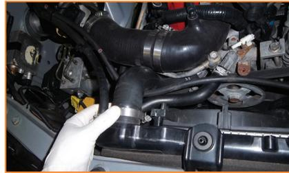
4. Remove the coolant catch tank by loosening the (2) 10mm bolts that hold the tank to the fan shroud.
