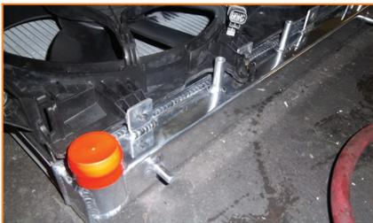
2. Install the lower rubber bushings onto the lower mounting pegs of the Mishimoto radiator and install radiator into engine bay. Connect the lower radiator hose and the 2 cooling fan plugs that were disconnected earlier.
