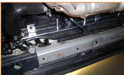
3. Install the upper coolant hoses. For 2004 and 2005 model year vehicles, plug the radiator cap bleed off tube. For 2006-2008
