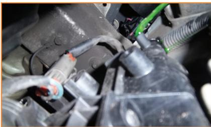
2. Unplug the other fan connector for the second radiator fan as well as the lower radiator hose.
