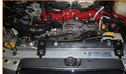
4. Install the coolant overflow bottle back onto the fan shroud and appropriate lines. Install the upper mounting brackets with the rubber insulators.
