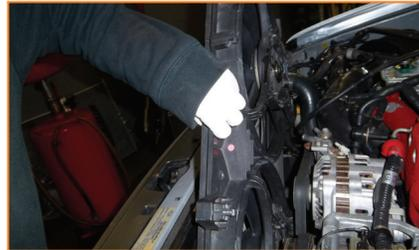
6. Remove the upper radiator support brackets. Qty 2-10mm head bolts.
