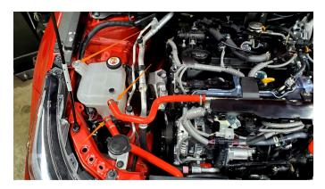
4. Install the hoses that were disconnected in Step 2 onto the Mishimoto expansion tank and secure them with the two (2) supplied worm gear clamps.
