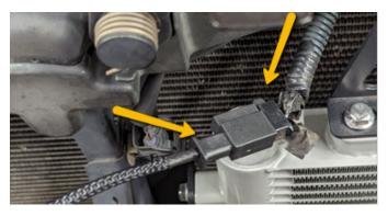
6. Plug the other end of the horn harness extension into the horn.
