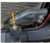
**10.** Locate the hole next to the driver-side headlight in the radiator support. Feed the transmission hose through the hole until the rigid section is centered in the hole. The end with a single hose should be in the engine bay. (Headlight removed for clarity)
