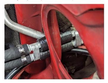
11. Attach hoses to the transmission cooler and secure them with provided hose clamps.
