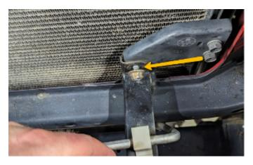
5. Plug the horn harness extension into the horn harness.
