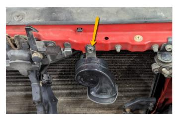
3. Disconnect the wiring harness from the horn, then remove
