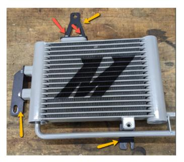
9. Align the top bracket with the threaded hole where the horn was originally located. Align the slot in the lower bracket behind the M6 nut that you left loose. The left side bracket aligns with an unused threaded hole below the ambient temperature sensor. Use the supplied M8 and M6 bolts to bolt the transmission cooler to the vehicle. Tighten all hardware.
