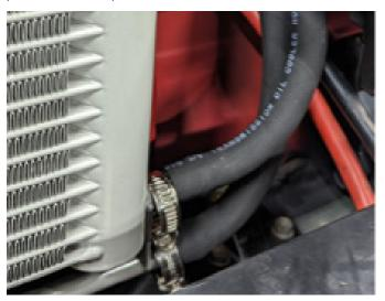
12. Remove the upper transmission hose from the radiator and reinstall it on the end of the hardline. Reuse the factory spring clamp to secure the hose.
