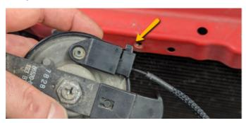
7. Locate the unused threaded hole on the upper radiator support.
