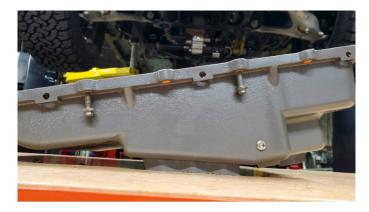
**04.** Install the Mishimoto pan onto the transmission. Torque the bolts to the specifications and in the sequence shown below.
