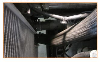
**6.** Remove (3) 12mm bolts for the thermostat housing and remove housing. Remove thermostat.
