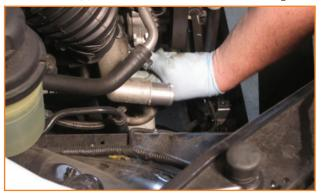
**3.** Reinstall the lower hose. Reinstall and tighten the negative terminal of the battery. Refill coolant, check for leaks, and bleed out air by turning the vehicle on and squeezing the upper and lower radiator hoses.
