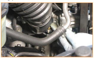
2. Reinstall the (3) 12mm bolts for the thermostat housing.
