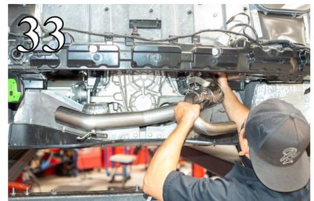
**WARNING:** Use extreme caution during installation. Torque all fasteners according to manufacturer's torque values and tightening sequence. **DO NOT** use impact tools to tighten fasteners on Borla Performance Exhaust Systems. Use of such tools may result in bent flanges or gasket contact areas leading to exhaust leaks.
