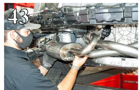
38. Front flange nut installation pictured (fig. 39). Do not fully tighten the nuts yet.
