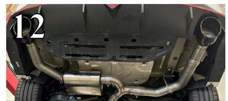
**WARNING:** Use extreme caution during installation. Torque all fasteners according to manufacturer's torque values and tightening sequence. **DO NOT** use air impact tools to tighten fasteners on Borla Performance Exhaust Systems. Use of such tools may result in bent flanges or gasket contact areas leading to exhaust leaks.
