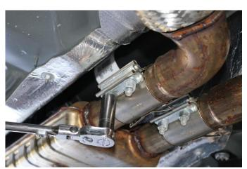
Use a flat head screw driver to pry open the locking spring tab on both of the sleeve clamps at the cat-back connection point.
