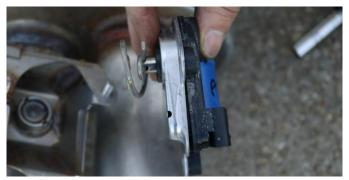
7. Use a 3/8" drive ratchet and a 10mm socket to remove the three nuts on each actuator. Remove the actuators from their valve assemblies. Place the actuators in a safe location to be used during Install Step 11. Install the hardware back onto the studs or store in a safe location since they will not be re-used during installation.
