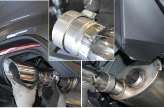
10. Install one 3" clamp on passenger non-valve tip assembly inlet pipe with nut towards the inside of the vehicle, bolt horizontal and towards the top. Slide tip assembly over muffler outlet pipe and tighten clamp using a ratchet and 15mm deep socket until tip assembly is snug on muffler outlet pipe. Repeat on driver side.
