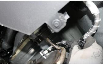
Reposition the driver and passenger valve actuator harnesses over their corresponding muffler hangers.
