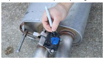
6. Place a piece of tape on each exhaust valve actuator and label them "D" for driver and "P" for passenger side.
