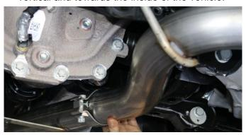
**6.** Slide the rear hanger into the passenger rear hanger grommet located just inside the passenger side tip cut out. Slide the muffler inlet pipe over the passenger side X-Pipe outlet.
