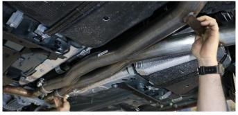
3. Install two 3" clamps on the CORSA X-Pipe inlets so the nut is towards the ground, and the bolt is vertical and towards the outside of the vehicle. Slide X-Pipe inlets over the adapter outlets. Position X-Pipe so its cross-brace is at the rear and facing the ground. Center X-Pipe outlets around the rear differential. Tighten clamps using a ratchet and 15mm deep socket until X-Pipe is snug on the adapters.
