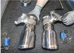
11. Confirm the spring wire form is correctly positioned on the passenger side stock valve actuator from **Removal Step 7**. Position and install passenger valve actuator onto the CORSA passenger valve tip assembly. Confirm that the spring wire form is located within the grooves of the valve assembly.
