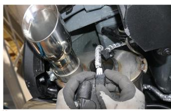
14. Connect the driver side harness into the actuator mounted to the driver valve tip assembly by pushing the plug until you hear a click, followed by the white locking clip.
