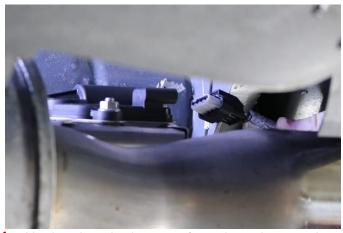
Unplug the wire harness from the exhaust valve actuators located on the inner most driver and passenger tips. To release the plug, slide the white locking clip away from the actuator, press down on the clip and slide the plug away from the actuator.
