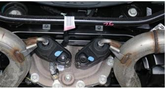
**4.** Use a 3/8" drive ratchet and 13mm socket to remove the bolt holding the driver side hanger grommet assembly. Save bolt for **Install Step 7**. Push up slightly on the exhaust and slide the hanger grommet assembly rearward to free it from the rear suspension sub-frame. Rotate the hanger grommet assembly a minimum of 90° so it will not interfere with the rear suspension sub-frame. Repeat for passenger side.
