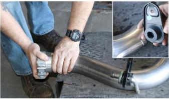
from **Removal Step 9** onto the front hanger of the CORSA passenger muffler assembly in the same position as it was installed on the stock exhaust. Install one 3" clamp on the muffler inlet pipe with the nut towards the ground, the bolt vertical and towards the inside of the vehicle.
