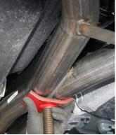
4. Tighten the clamps at the front of the X-Pipe using a ratchet and 15mm deep socket until the X-Pipe is snug on the adapters. Place a jack stand or similar device under the X-Pipe for support.
