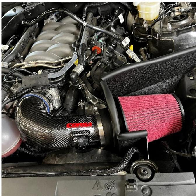
**9.** Attach the filter to the opposite end of the duct and tighten all clamps using an 8mm socket.
