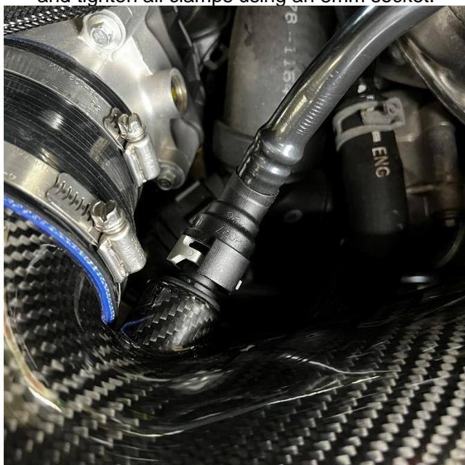
**11.** Re-attach the breather line to the larger quick disconnect fitting.
