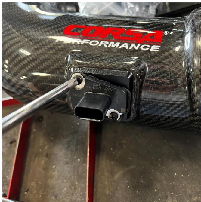
2. Install the MAF sensor and gasket on to the duct.
