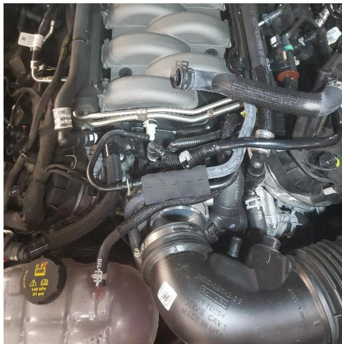
**10.** Pull duct from throttle body.
