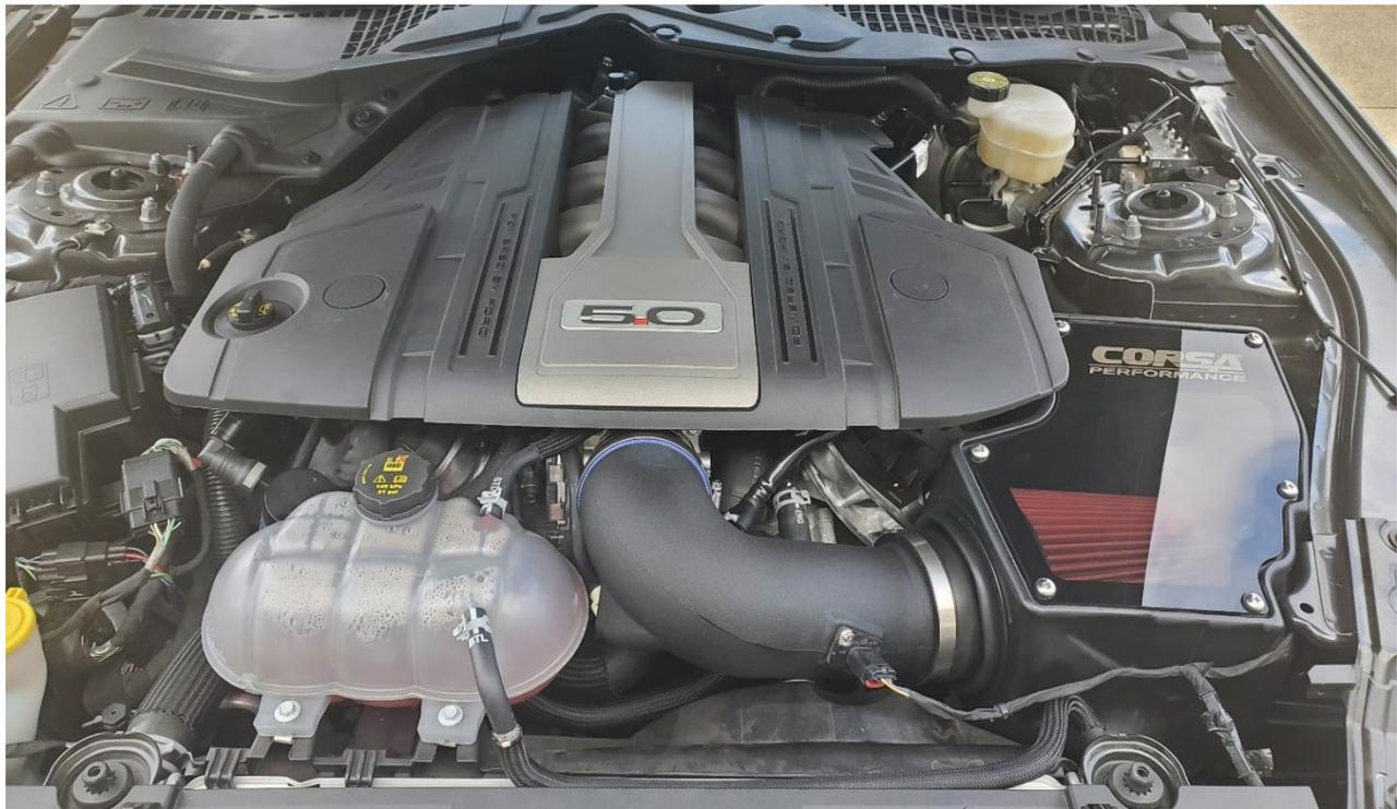
**14.** Install engine cover re-using factory hardware.
