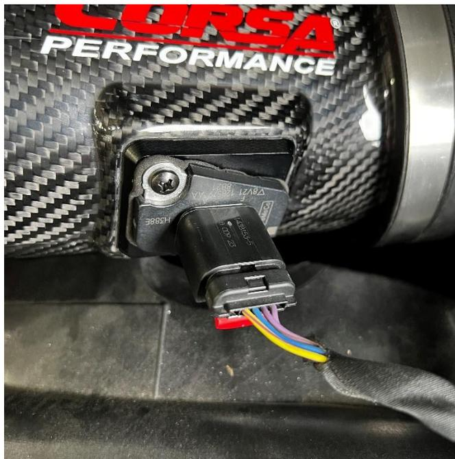
**10.** Clip MAF sensor wiring harness back into the MAF sensor in the correct orientation
