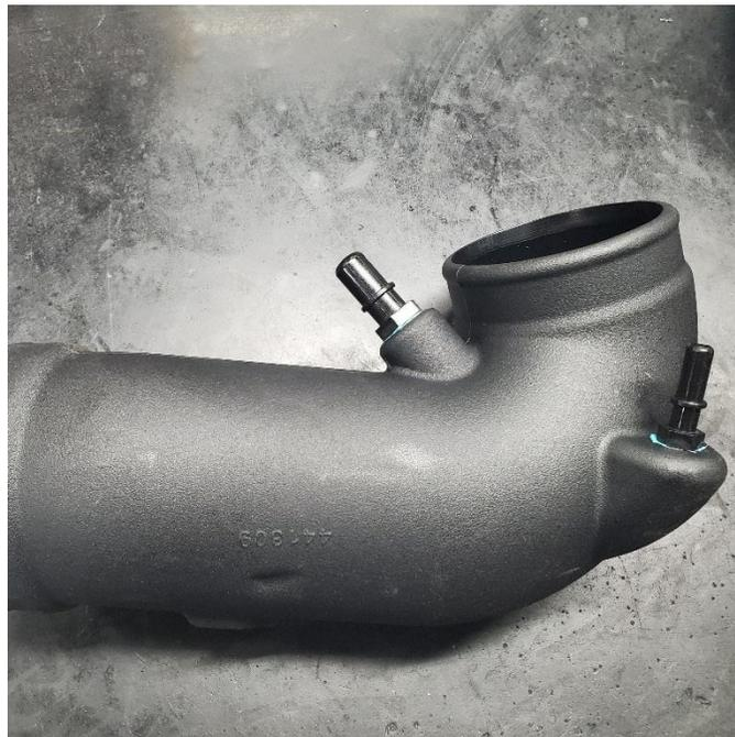
2. Install large fitting in threaded hole on inside of bend (left fitting in picture). Install small fitting in threaded hole on outside of bend (right fitting in picture). Tighten fittings until completely seated but do not overtighten.
