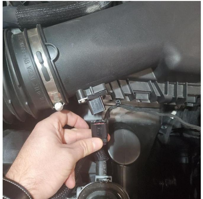
**4.** Unclip wiring harness from MAF sensor.
