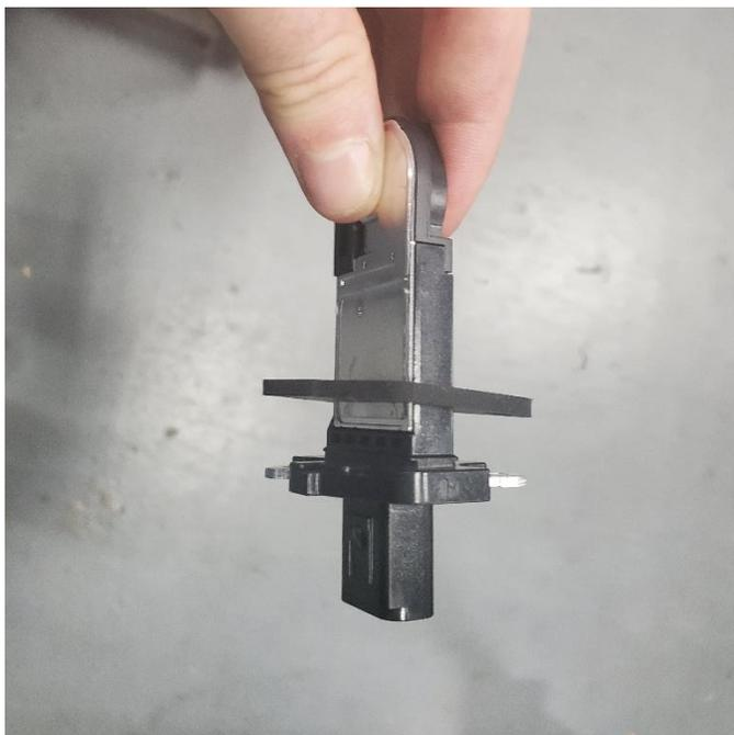
3. Place the included MAF gasket onto the MAF sensor.
