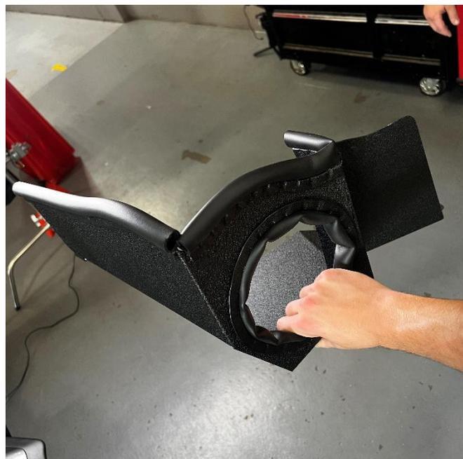
4. Use the provided seal trim by adding it along the top of the heat shield and around the filter opening. You may need to cut the trim as needed
