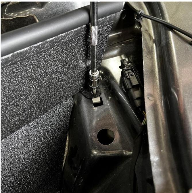
**7.** Use the 10mm bolt that was removed in removal step 14 to secure the shield.
