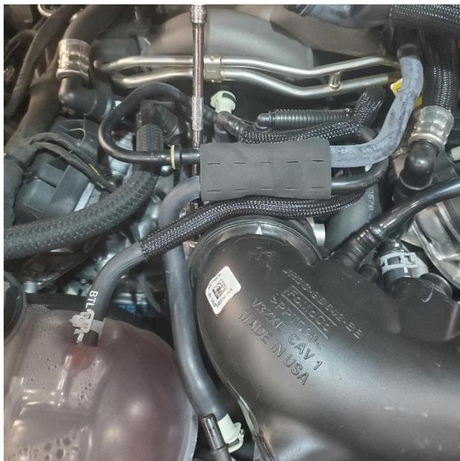
**9.** Using 7 mm socket loosen throttle body clamp.
