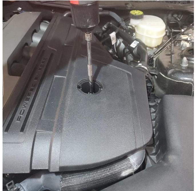
**2.** Using a 10mm socket remove the two nuts securing the engine cover.
