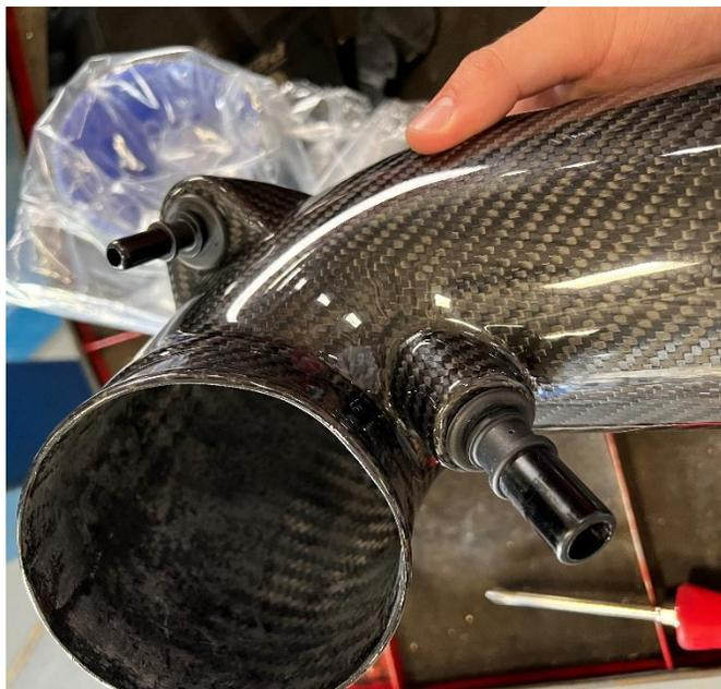
1. Install the provided grommets and fittings to the air duct.
