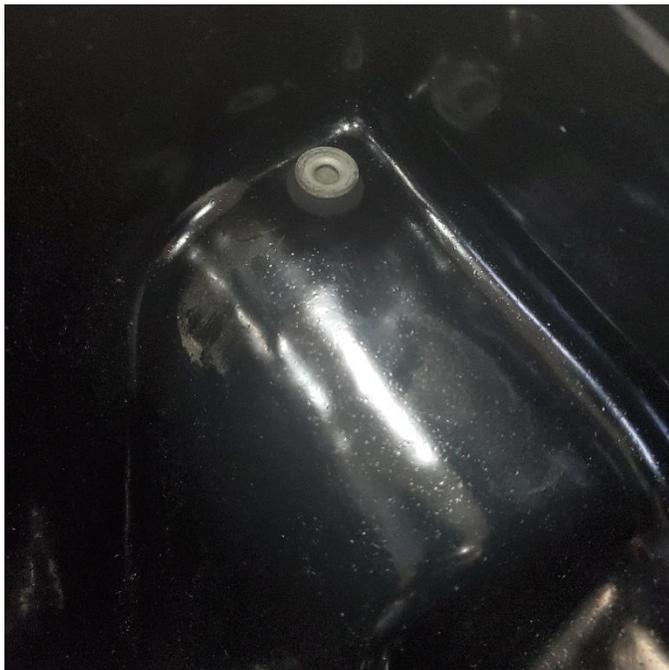
1. Insert grommet and bushing from removal step 20 into CORSA air box.
