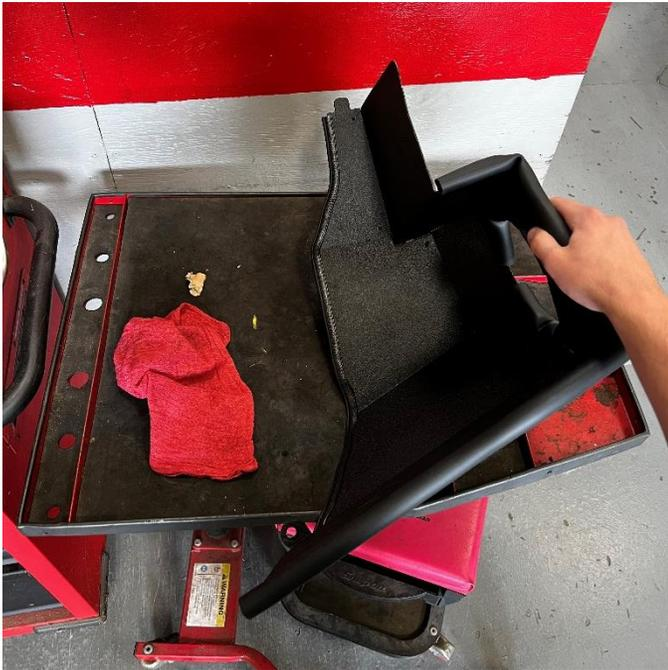
**5.** Use the smaller seal trim by attaching it to the back side of the shield. You may need to cut the trim as needed
