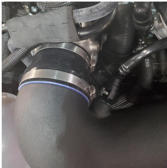
**9.** Install filter band clamp onto filter. Install air duct into position in vehicle with #56 clamp on smaller end of reducer pushing reducer onto throttle body until seated. Tighten all three clamps using 8mm socket.
