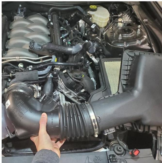
**12.** Remove duct with upper airbox.
