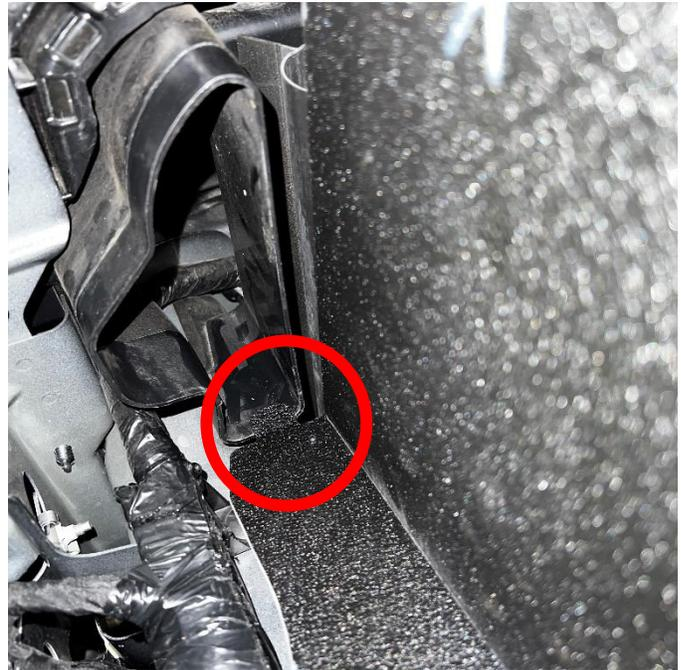
**6.** Insert the shield into the engine bay. The tab on the end of the shield will sit on top of the inlet tube.
