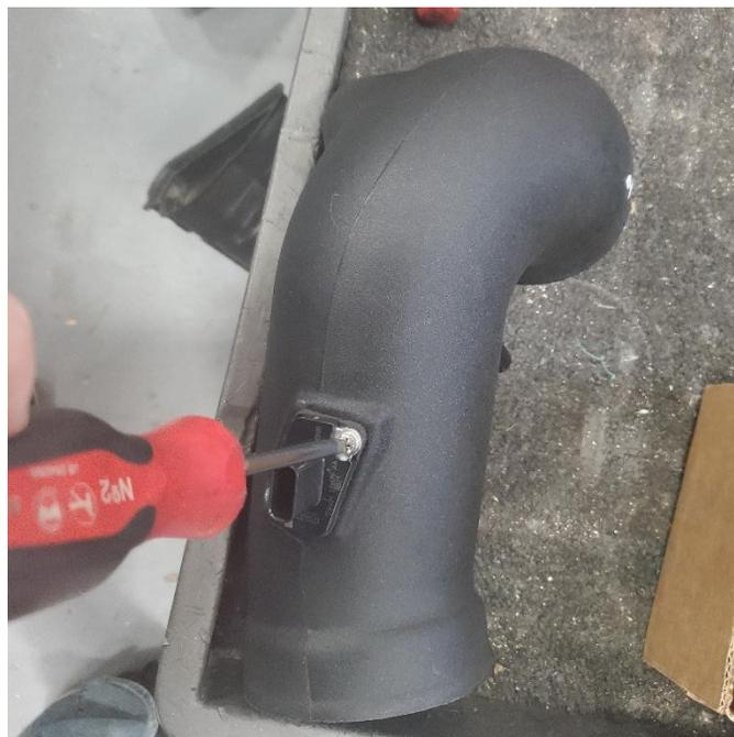
4. Install MAF sensor into CORSA air duct and secure with included screws.
