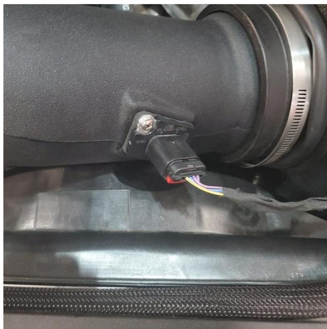
**12.** Plug MAF sensor wiring harness into sensor. Press red locking tab in to secure.
