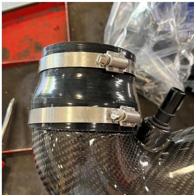
3. Attach the reducer sleeve and clamps to the smaller side of the duct.
