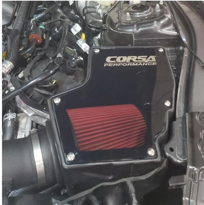
**13.** Install lid onto air box with lid screws. Do not over tighten screws.
