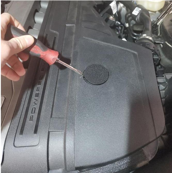
**1.** Remove the two covers concealing the engine cover mounting nuts.
