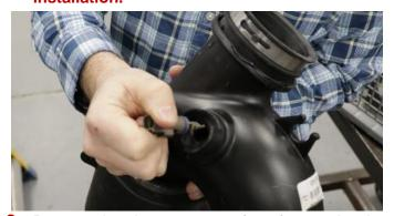
Remove the air temp sensor from factory duct by gently lifting tab and rotating counterclockwise until it stops then pulling straight out.
