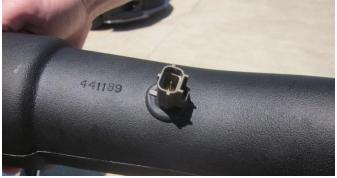
Locate air temperature sensor from removal step 9 and CORSA air duct. Install sensor into grommet with tab facing the closest end of air duct.
