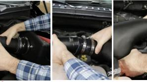
13. Install air duct into vehicle by placing the hump hose onto the filter adapter, then place reducer onto the upper stock inlet. Rotate duct down and into the straight sleeve.
