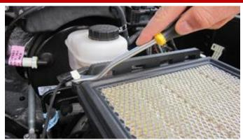
**5.** Remove the three plastic wire retention clips from back of factory air box using a trim removal tool.
