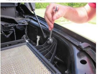
Use a ratchet and 13mm socket or wrench to remove the bolt holding the air box to the vehicle.
