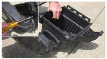
8. Remove the bolt attaching the scoop to factory air box using a ratchet and 8mm socket. Remove the factory air scoop from the bottom of the air box
