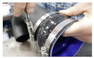
10. Locate the hump hose and two # 64 clamps. Install the hump hose and one clamp onto the air duct inlet end and tighten clamp using a flathead screwdriver or ratchet and 8mm socket. Loosely place other clamp on hump hose.
