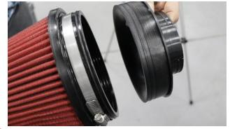
Locate filter and filter adapter and insert the filter adapter into filter. Tighten clamp enough that it won't fall off filter but leave loose enough to rotate.
