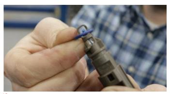
**10.** Remove O-ring from the temp sensor.
