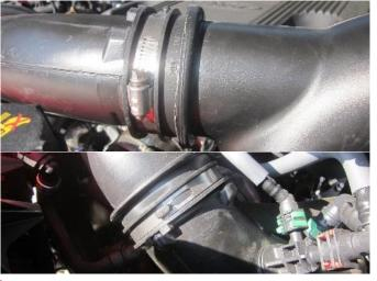
Loosen the clamps on the top and bottom intake tubes using a ratchet and 7mm socket or flathead screwdriver.
