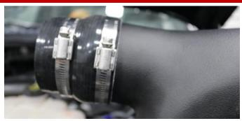
12. Locate reducer, #56 clamp and #48 clamp. Install large end of reducer and # 56 clamp onto upper outlet of air duct. Tighten clamp using a flathead screwdriver or ratchet and 8mm socket. Loosely place #48 clamp onto reducer.
