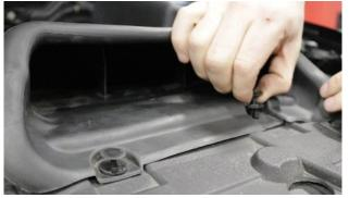
**5.** Locate the air scoop retaining clips from removal step 6 and attach factory scoop.
