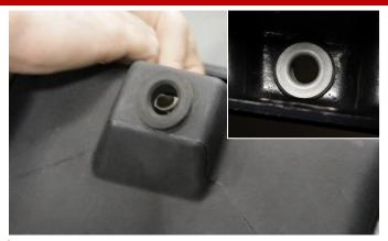
Locate the CORSA air box, and the factory grommet and metal bushing from Removal Step 7 and install grommet in air box then the metal bushing into grommet from inside box.
