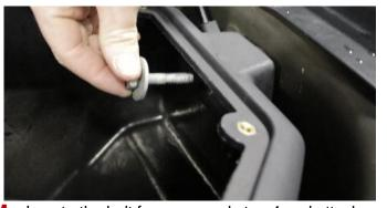
Locate the bolt from removal step 4 and attach the CORSA air box to the inner fender using a ratchet and 13mm socket.
