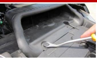
6. Remove the two plastic clips from the factory air scoop using a trim removal tool.
