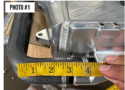
Suggested cut measurement approx. 4" from inside radius for top fitting/approx. 3" for bottom fitting
