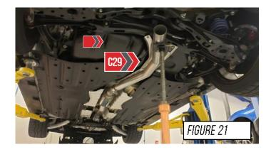
When installing your AWE rear section you will need to use the appropriate exhaust hanger locations.
