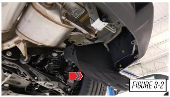
Remove the 3 bolts from the OEM exhaust flange that attaches the front pipe to the OEM downpipe, as shown in **Figure 4.**
