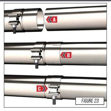
Next, install the tri-tip merge (Part C35) onto the exhaust system using one of the 3 inch exhaust clamps.
