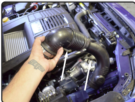
6. Remove the OEM vibramount from vehicle! Now lift up and remove the stock intake tube from the vehicle.
