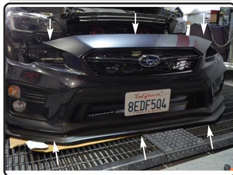
7. Loosen and remove the front bumper cover for the installation of the injen intake system.
