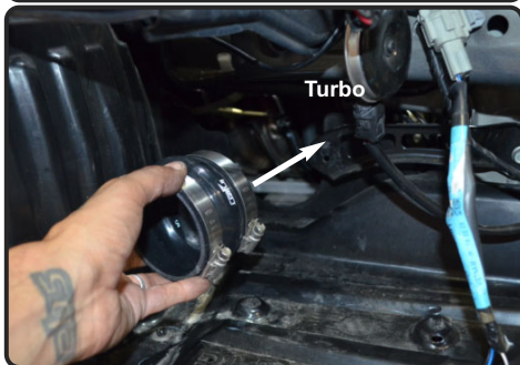
10. Install the provided 3" hump hose with clamps provided to the turbo. Tighten the clamp on turbo side only.
