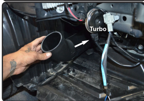
11. Install the lower intake tube and attach to the 3" hump hose and position. Do not tighten.
