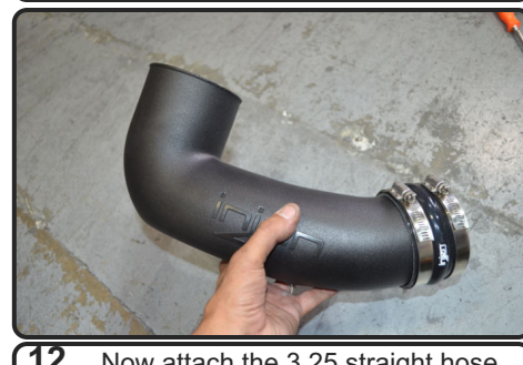
12. Now attach the 3.25 straight hose to the upper intake tube with clamps provided. Tighten the clamp on upper intake tube only.
