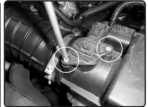
4. Loosen the 2 screws holding in the MAF sensor and remove. Save screws for later install.
