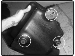
**12.** Make sure the grommets are seated and secured.
