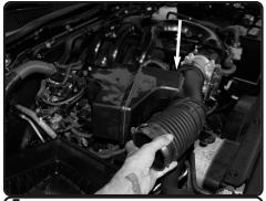
**5.** Now lift up and remove the stock intake tube from the vehicle.
