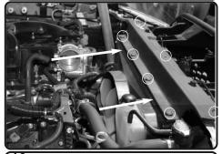
**10.** Loosen and remove the 7 push clips holding in the radiator plastic shroud and remove. Save 2 push clips for later install.
