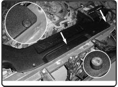
17. Position the scoop and make sure the smaller holes are used for the 2 push clips from step 10. The 2 hood bushings will go through the scoop.
