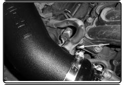
**22.** Re-connect the crank case line to the injen intake tube.
