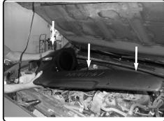
**15.** Install the air box assembly into the vehicle and position.
