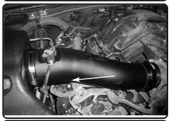
**23.** Tighten all clamps using 8mm ut driver. Re-install the engine cover.
