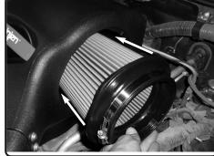
**18.** Insert twist lock filter to the air box.
