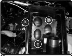
**6.** Loosen the 3 bolts holding in the lower part of the airbox.
