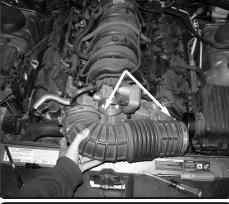
**6.** Remove the OEM intake tube out of the vehicle.
