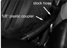
**20.** Install the provided 17mm hose and plastic coupler to the stock crank case hose. Connect the two and secure to the intake tube
