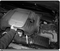
**2.** Lift up and remove engine cover.
