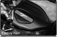
11. Install the air box assembly into the vehicle. Secure using OEM screw. Make sure the nipple fitting on back side of injen airbox is seated in the OEM grommet on fender well.
