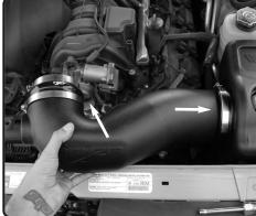
**15.** Install the intake tube assembly into the vehicle and position.
