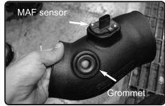
**12.** Install the provided crankcase grommet to the hole cutout on the tube.
