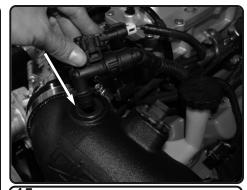
**15.** Now install the crankcase line into the grommet.
