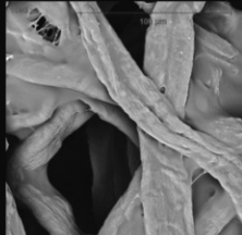
Existing media without Injen SuperNano-Web Technology
