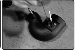
11. Secure and tighten the MAF sensor using provided M4 button head screws.
