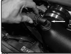
**18.** Re-install the sound tube from step 5 and secure to grommet.
