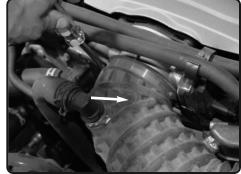
**3.** With 8mm nut driver, loosen the clamp on the throttle body and pull back tube.
