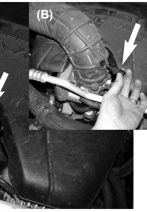
Figure 6(B) Firmly pull air temp sensor out of factory air duct. This sensor will be re-used later.
