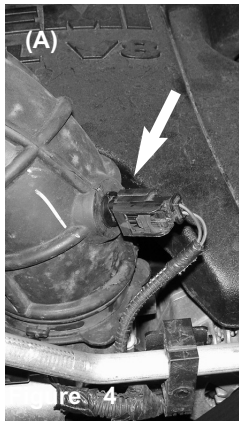
Figure 5(A) Stock air temp sensor on factory air duct.
