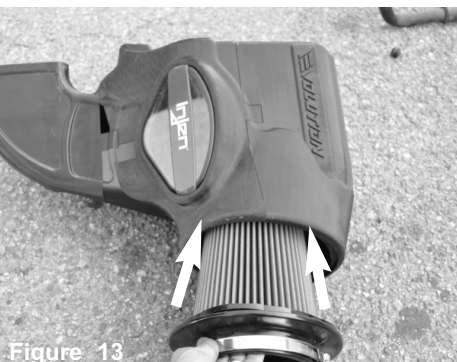
Figure 13 Remove the factory grommets from the OEM air box and install to the new injen air box.
