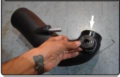
**11.** Install the temp sensor adaptor to the tube and secure using provided M4 button head screws.
