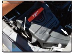
**8.** Install the air box assembly into the truck and position the air box to the studs from the OEM air box. Make sure the front of air box is seated properly.
