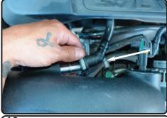
**16.** Reconnect the crank case harness to the machined fitting. You will hear a clicking noise once the harness is secure.
