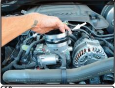
**10.** Install the provided 3.5" hump hose with clamps to the throttle body. Secure and tighten on the throttle body only.
