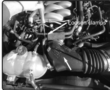
**2.** Loosen the clamp on the throttle body using 7mm nut driver or flat head screwdriver.
