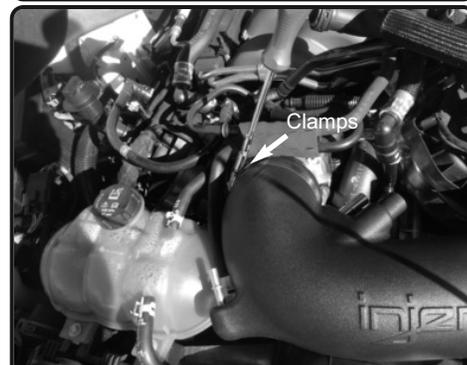
**8.** Adjust the tube for best fitment and then secure the clamps.
