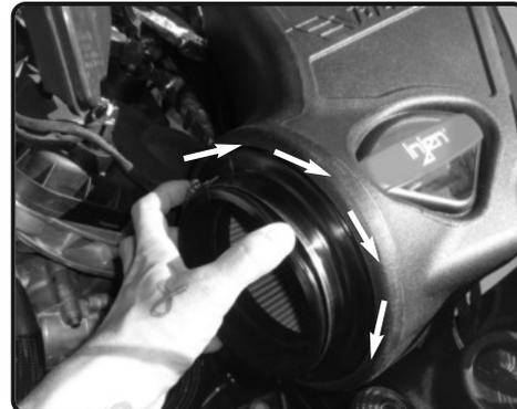
**4.** Once seated, Secure the twist lock filter by rotating in either direction 1/4" turn until filter locks into place.
