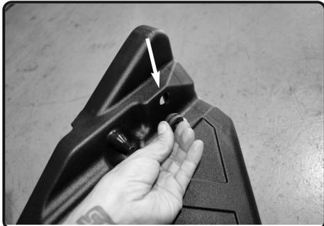
**9.** Install the smaller grommet and spacer washer from figure 8 into the 1/2" hole on the Injen lower air box assembly
