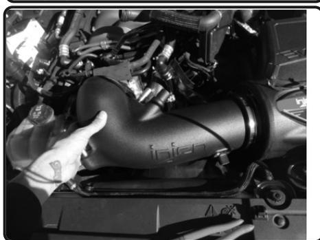
**7.** Place the Injen intake tube onto the throttle body and twist lock filter. Adjust the tube for best fitment and then secure the clamps.
