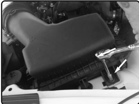
**5.** Remove the 10mm bolt from the OE air box assembly.
