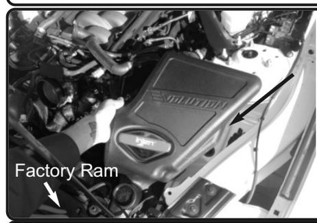
**11.** Drop the Injen lower air box assembly into the factory air box location. The front ram air should just slide into the Injen air box.
