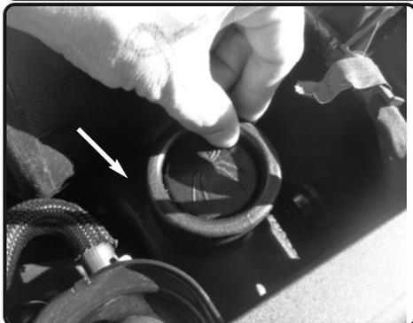
**5.** Install the provided filter monitor plug into the slot. (Sold separately is our injen filter monitor see injen.com for more info)
