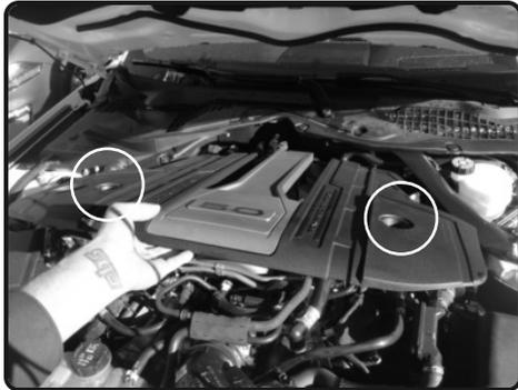
**1.** Stock intake system shown. Loosen the 2 nuts holding in the engine cover. Remove engine cover.
