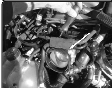
**6.** Install the urethane step hump hose to the throttle with clamps provided and tighten clamp on throttle body only.
