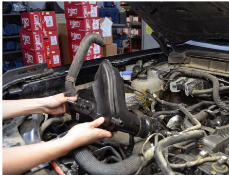
17. Remove the OEM intake tube from the vehicle.
