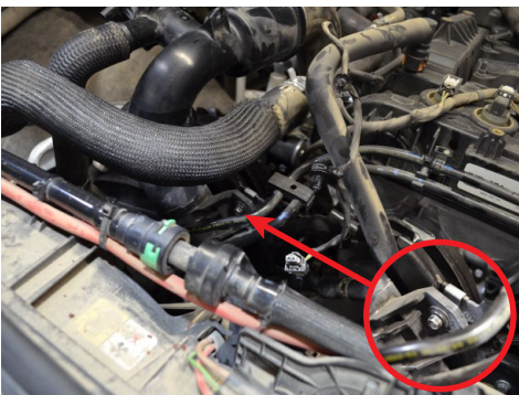
10. Remove the bolt securing the bracket on the intercooler pipe.
