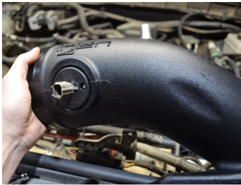
26. Install the IAT sensor to the adapter from figure 24. Once fully seated, rotate the sensor to secure in place.
