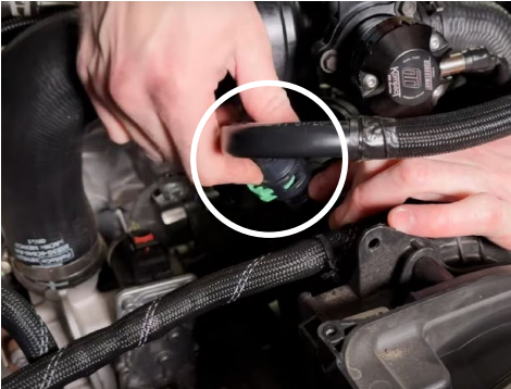
4. Lift up on the green tabs, then push the clip back to release the lock. Detach the crank case line from the fitting on the OEM intake hose.
