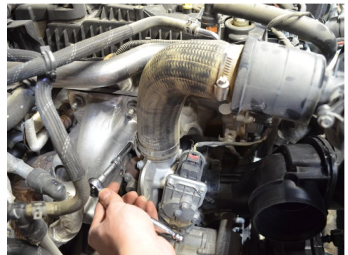
9. Loosen the clamp that's securing the intercooler hose to the turbo.
