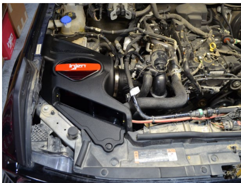
35. Reinstall the OEM intercooler pipe by following step 8-13 in reverse order. Once complete, ensure all nuts, bolts, and clamps are properly secured.
