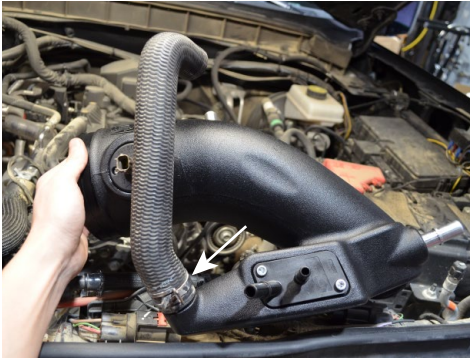
28. Install the OEM diverter valve hose onto the injen tube. Secure the hose with the OEM tension clamp.
