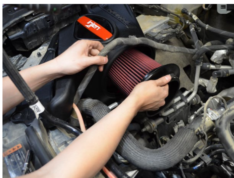
23. Install the twist lock filter on to the Injen air box. Once seated, rotate the filter a 1/4 turn in either direction so the filter can lock into place.
