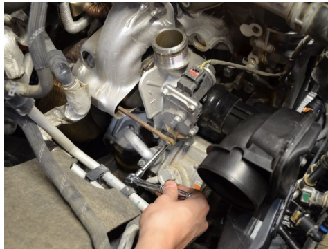
16. Loosen the clamp securing the OEM intake tube to the turbo.
