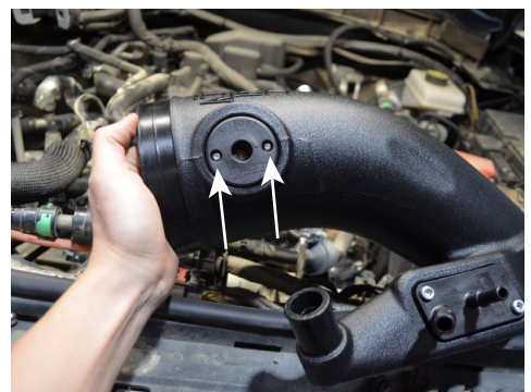
24. Secure the temp sensor adapter onto the Injen tube using the provided M4 bolts.
