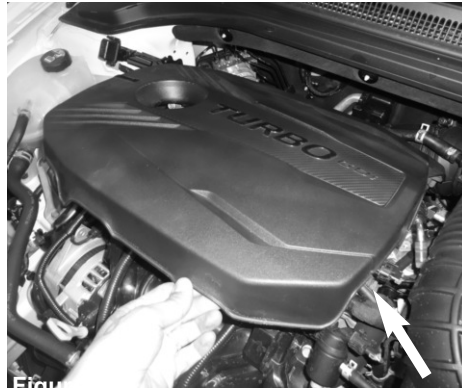
Figure 4 Firmly lift up on the engine cover and remove the engine cover from the engine bay.
