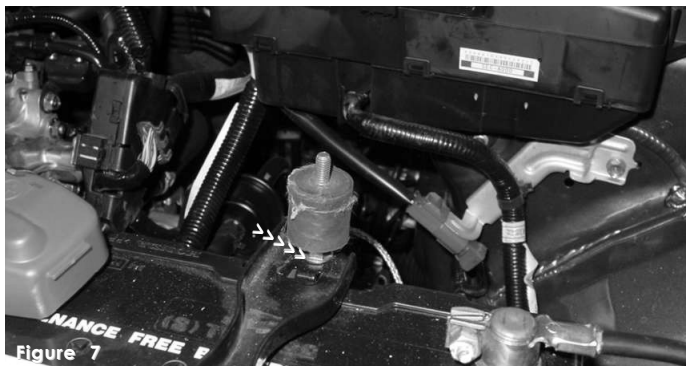
Figure 7 Take the male/female vibra-mount and screw it over the threaded battery post. Do not bottom out the vibra-mount a full 20 turns will be more than enough.
