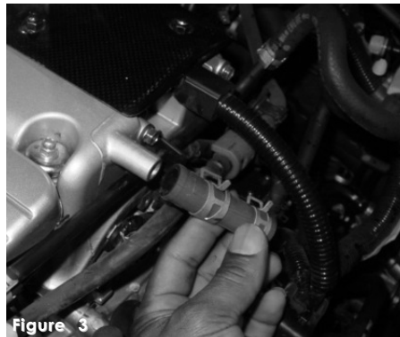
Figure 3 Remove the breather hose from the PCV pipe and press it over the crankcase port. Use the stock hose clamps to secure the lines in place.
