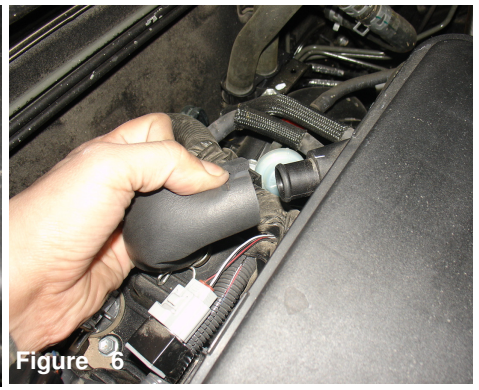
Figure 6 Remove crank case line from stock intake system.
