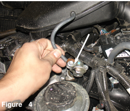
Figure 4 Pull back the vacuum line from the actuator. Leave connected to box so you will not lose this piece.
