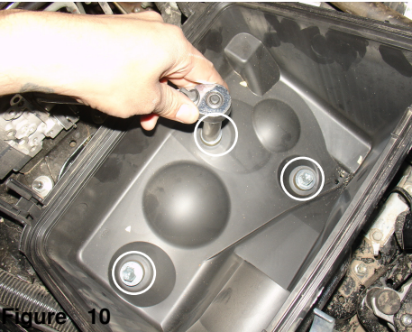
Figure 10 Loosen the 3 bolts holding in the bottom half of the air box. Remove the bottom half of the air box.
