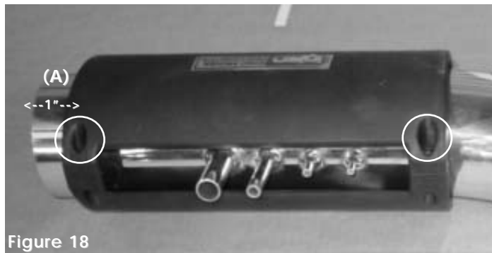
Figure 16 Each heat shield will take two rubber spacers that are pressed over the locating pins. Each end has two locating pins, the rubber spacer works best when it is pressed over the inner pins. This will create the desired gap between bends that may obstruct the shields clearance.
