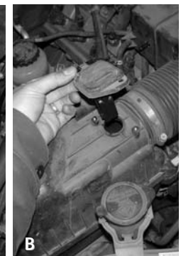
Figure 7 A Remove the vacuum switching valve line from the back side of the air duct. (Figure A). The entire vacuum switching valve line is removed and will be replaced with an Injen vacuum line later. (Figure B)
