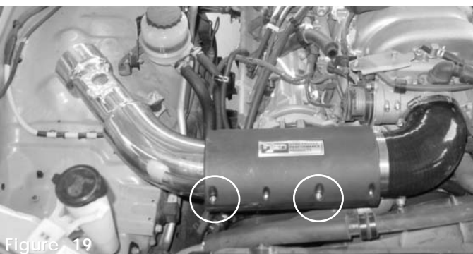
Figure 17 The window opening on the shields will face the vacuum ports. Lay the intake over the bottom half of the shield until it is snug in place. Take the top half of the shield and line up the bolt pattern to each other. Screw the m6 x m25 bolt into the press nuts seen on the bottom shield. See (A) and (B)
