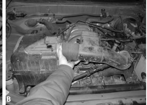
Figure 10 A Use a Phillips to unscrew the two screws holding down the MAF sensor. (Figure A) Then remove the MAF sensor from the factory air box cleaner
