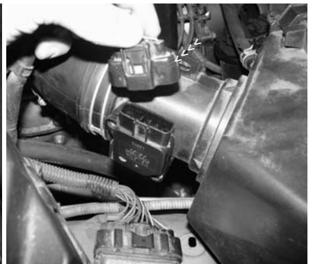
Disconnect the harness clip connected to the air mass sensor.
