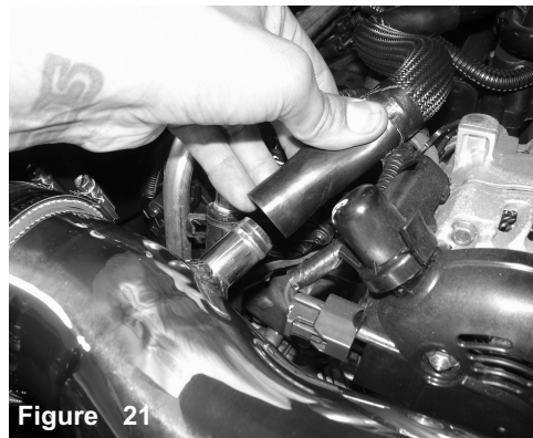
Figure 18 Install the grommet to the hole on the intake tube. This will be used for the temperature sensor.
