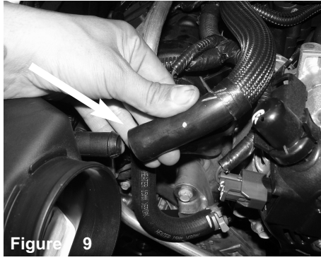
Figure 9 Pull back the crank case line from air box fitting.
