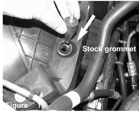
Figure 13 Now install the stand off stud to the factory grommet.
