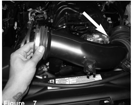
Figure 7 Carefully pull of the intake tube. Note: Temp harness still connected. See next step.
