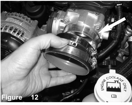
Figure 12 Now install the step hose with clamps provided to the throttle body. Tighten the clamp on the throttle body using 8mm nut driver.
