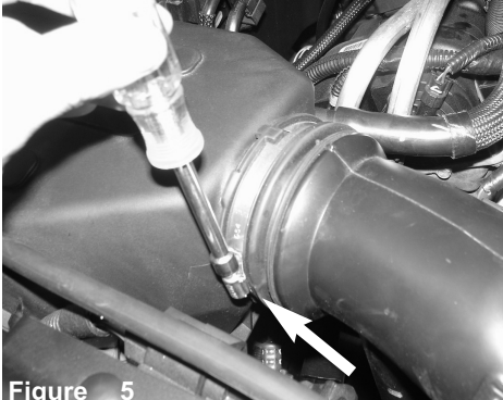
Figure 5 Loosen the clamp on the air box using 8mm nut driver.
