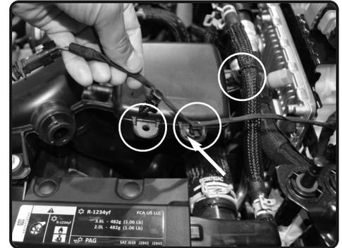
3. Pull back the temperature sensor harness from the intake tube.
