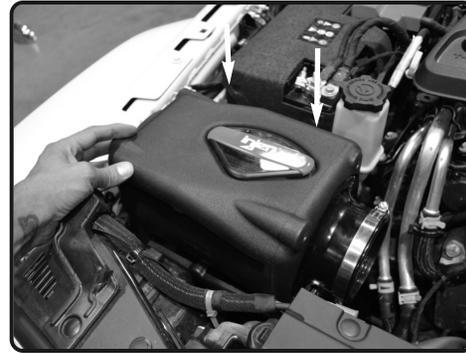
**14.** Powerslow box installed and seated properly.
