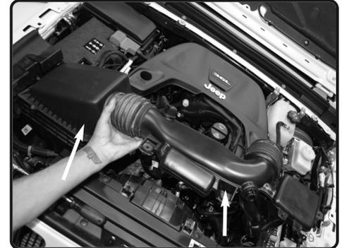
7. Now lift up and remove the air box assembly out of the vehicle.
