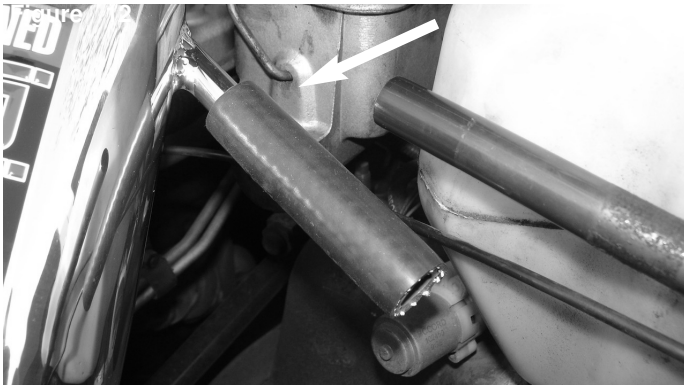
Now install the 12mm hose to the fitting on the intake tube. If not equipped use provided vinyl plug.
