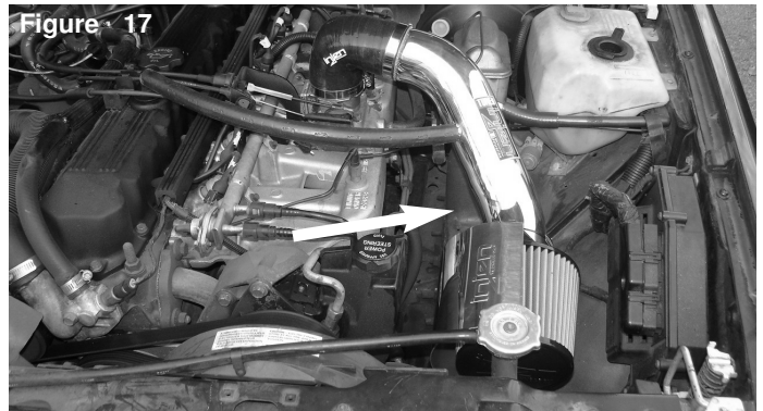
Position the intake so that it does not hit any lines or come close to anything. Your Injen intake installation is now complete. Check for any rubbing or any rattling. Tighten all clamps and re-tighten if necessary.
