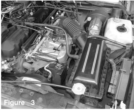
Figure 3 OEM intake system.
