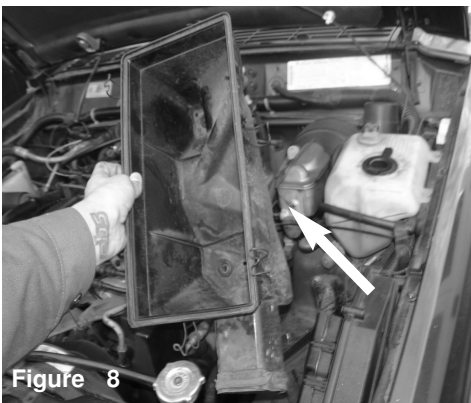
Figure 8 Remove the bottom half of the air box.
