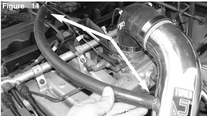
Install the 15mm hose to the engine and the fitting on the intake tube.
