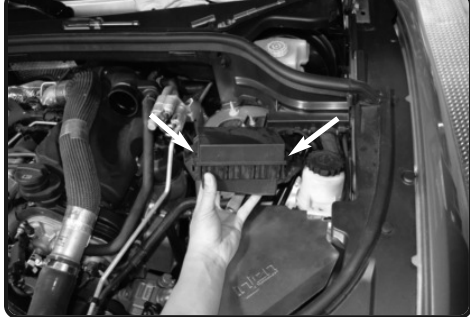
8. Remove the two 10mm nuts to move the fuse/relay box. This will give you more room to install the heat shield.
