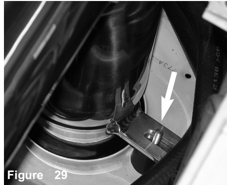
Figure 26 The intake is slowly rotated in clockwise position while lowering it into the resonator opening.
