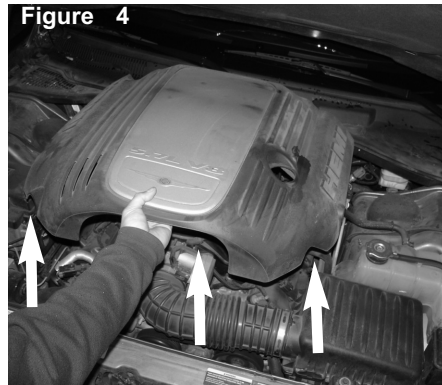
Lift up and remove engine cover.
